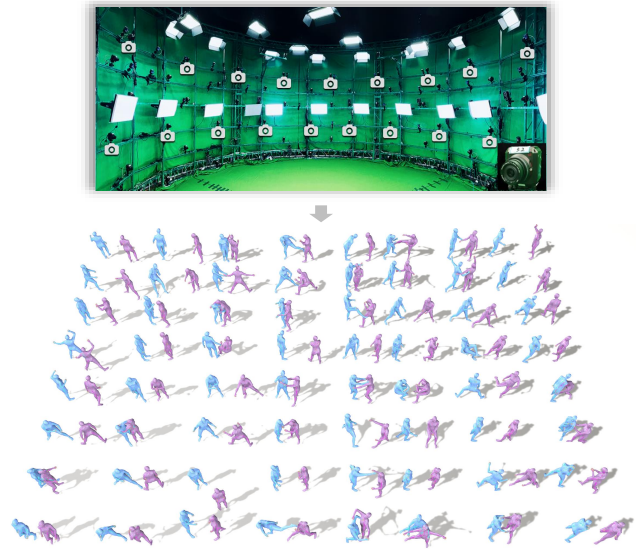
Fig. 2 Our motion capture studio (top) and our collected InterHuman dataset illustration (bottom). The system comprises 76 calibrated multi-view cameras. InterHuman covers a wide range of two-person interactions.
